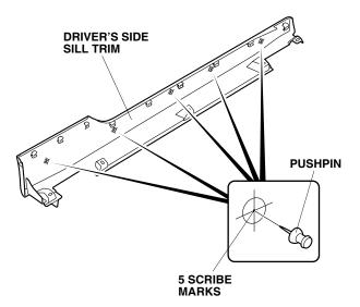
5. While wearing eye protection, drill the five holes made in the driver's side sill trim with a 3 mm drill bit, then finish with a 6 mm drill bit. Remove any burrs.
